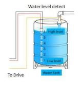
Level sensor used for automatic start and stop of motor in case of pumping to overhead tank
