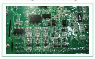
Bunit it braking unit for full power range of AC350.
