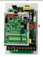
Innovation design with dual CPU to provide better performance and minimized fault occurs
