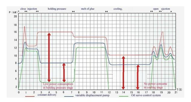
The injection molding machine power consume take up 75% of system total in traditional constant flow of IMM. It need difference flow and pressure during difference working stage of IMM such as mold close, injection, pressure holding, molding open. When the required over the setting pressure and flow, the flow and pressure will be adjusted by relief valve or proportional valve. this process call high pressure throttling. Up to 40-75% energy wasting during this stage.
